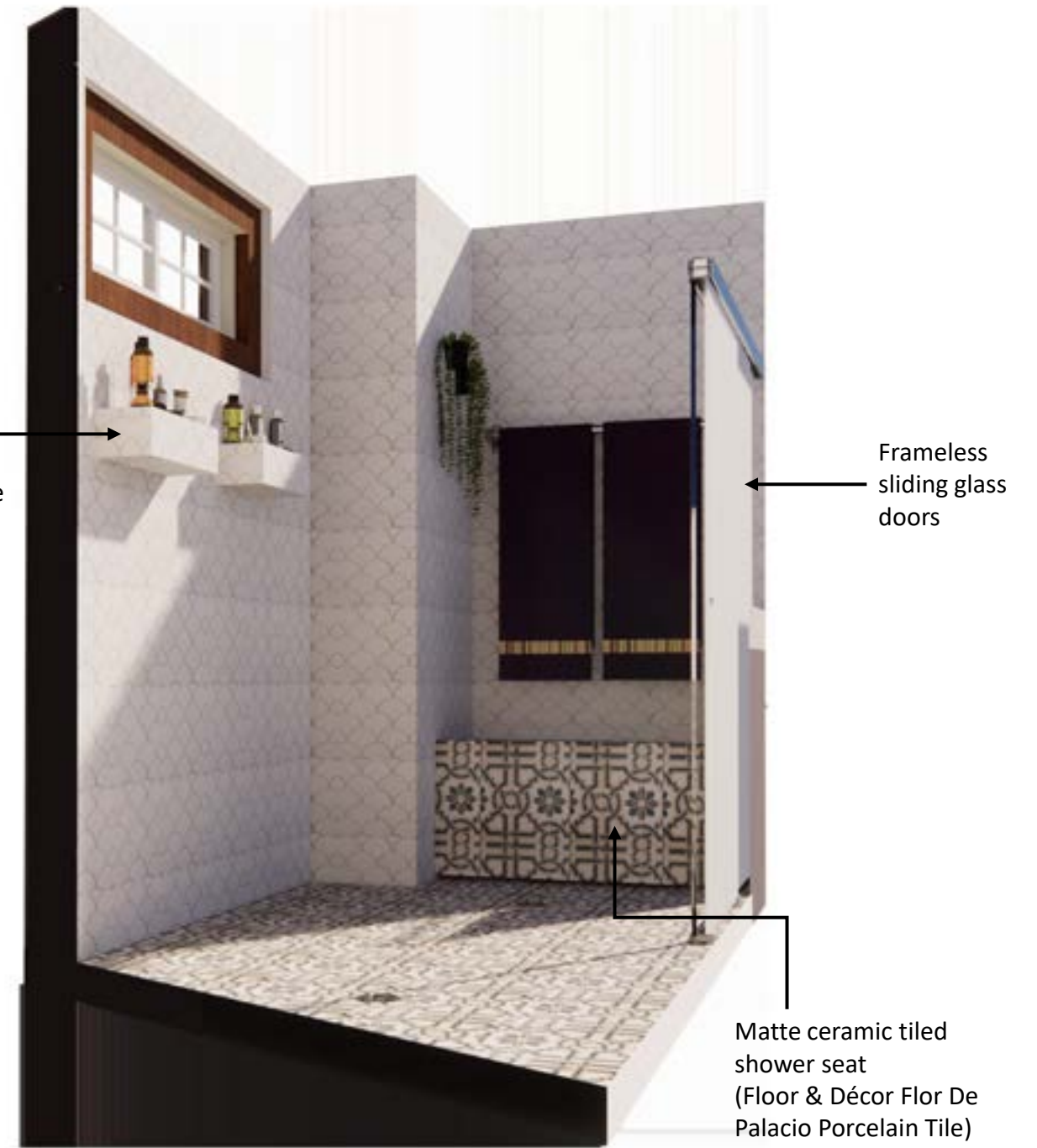
2 ND FLOOR MASTER BATHROOM SHOWER DETAIL
